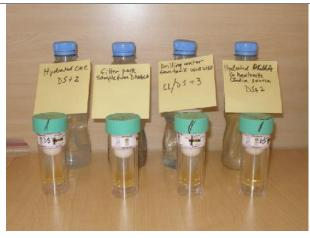
Using BART as field test to evaluate bio contribution of drilling fluid system components (Jordan)
