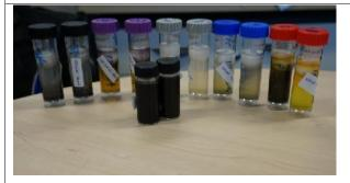
Reacted BART and PathoScreen tubes from an alluvial bore in Queensland
