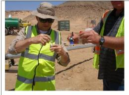
Inoculating using sterile outer tube – inverted tube center mixing indicator dye. Assembled tube R.
