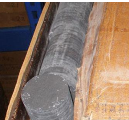
Fig. 3. Ohio shale core from Crawford County, Ohio (236 ft, OGS core collection)
