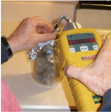
Fig. 2. Testing limestone rock for gas production
