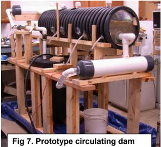
Fig 7. Prototype circulating dam drain model
