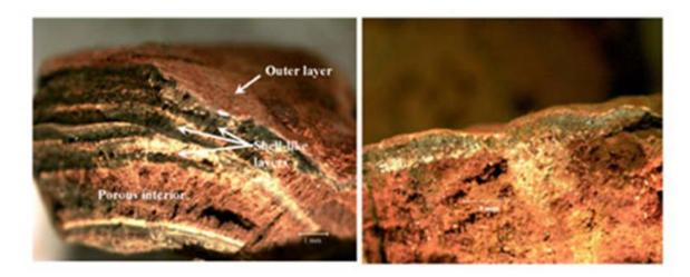
Fig. 10: Cross-sections of iron pipe (mild steel) corrosion tubercles (U.S. EPA)
